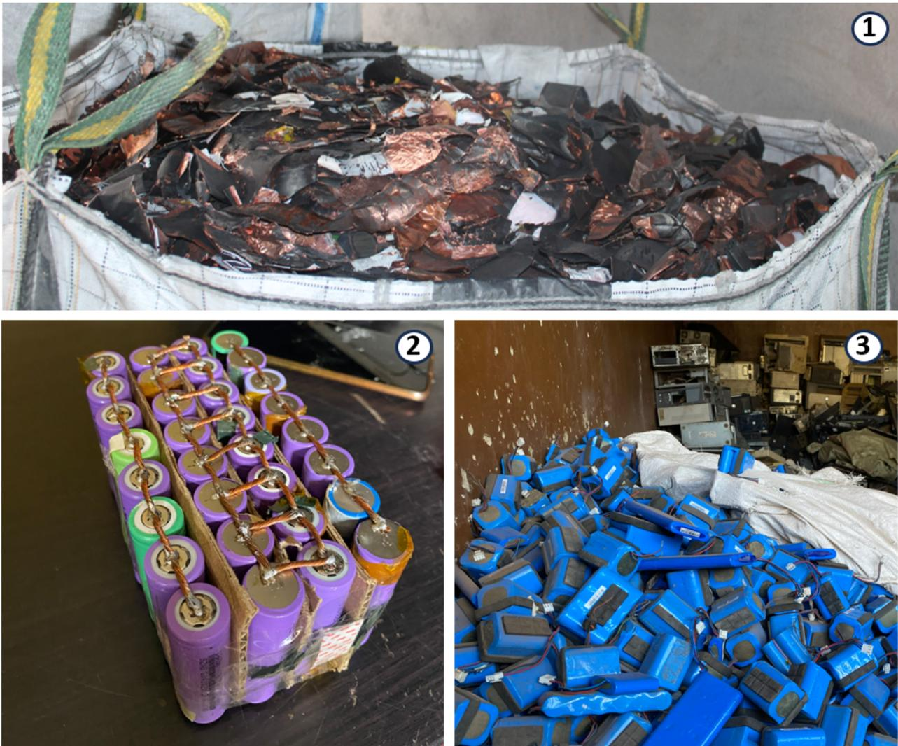
1: Copper foils from manual disassembly of Li-ion battery cells in a registered recycling company
